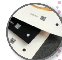
Vision3 camera reads black or white QR codes to instantly retrieve associated cut files
