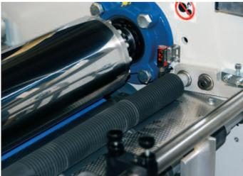
An infeed roller presents lightweight and digital output to the laminating and nip rollers where a missing sheet detector helps to prevent unwanted wraparounds.
