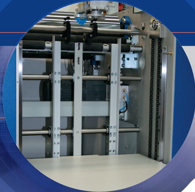
The suction feeder offers a deep pile for longer run work and is easily adjustable for a variety of different sheet sizes.
