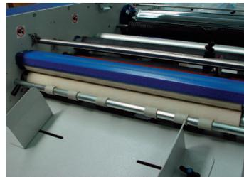
The adjustable burster automatically separates sheets up to B2 size. A cushion of air supports the sheet as it is delivered into the catch tray.
